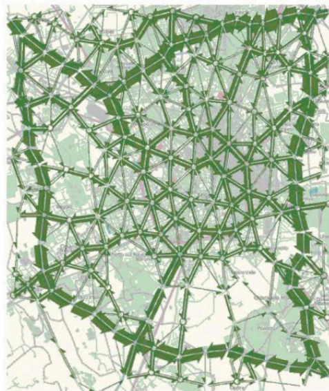
Figure 75: A flow map of the traffic in Milan. The trajectories are aggregated and only flows representing 50 or more trajectory segments are shown.
