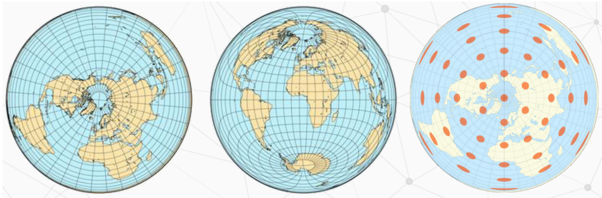
Figure 32: Lambert azimuthal equal-area projection with Tissot's indicatrix of deformation
